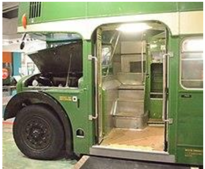
Passenger door and downstairs interior of a Bristol Omnibus Company Lodekka. Note the stairs directly in front of passenger door and bench seats over rear wheels.
