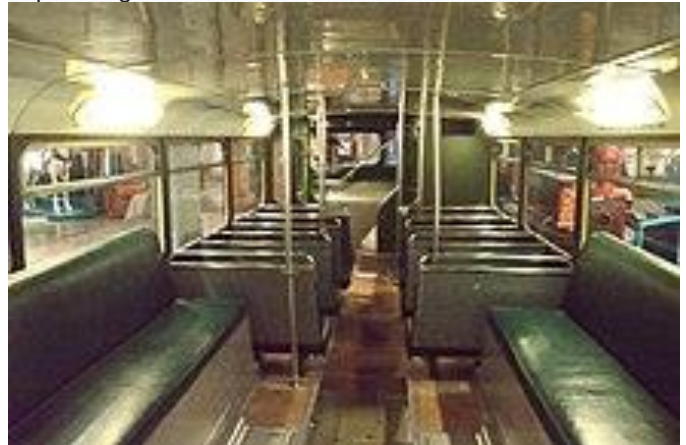
Passenger door and downstairs interior of a Bristol Omnibus Company Lodekka. Note the stairs directly in front of passenger door and bench seats over rear wheels.
