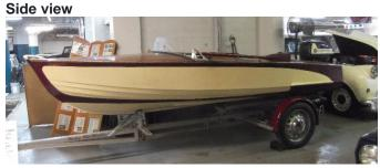
The Ski Masters were built at the Plymore Mills boatyard in Bridport, Dorset England by Aquaply Marine for Healey Marine Ltd. The hull is constructed of Aquaply African Marine plywood with the deck and seats made of African mahogany.
